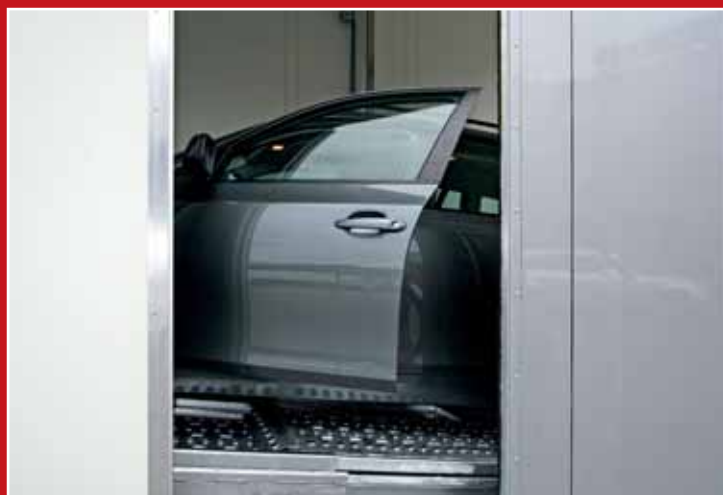
Due to the positions of the semitrailer's access doors you can comfortably open the doors of the loaded vehicles as well.
