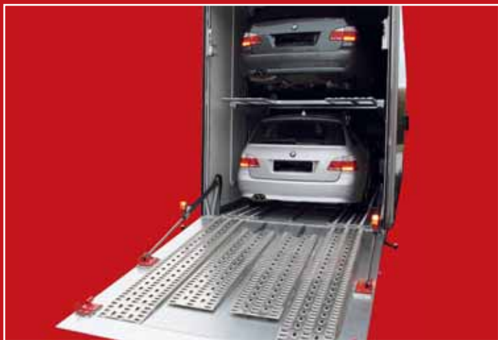
Using the tail gate as an access ramp offers simple operation and a perfect access angle.
