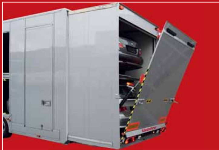
The telescopic rear end of the body increases the loading factor.
